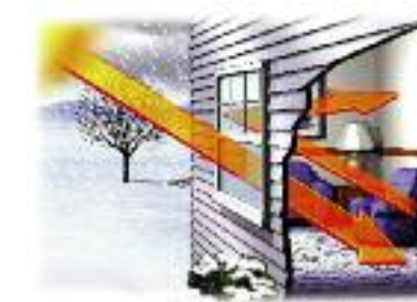
Low-E glass takes on a new duty in winter months. It lets warm solar rays into your home, while preventing indoor heat from escaping.
